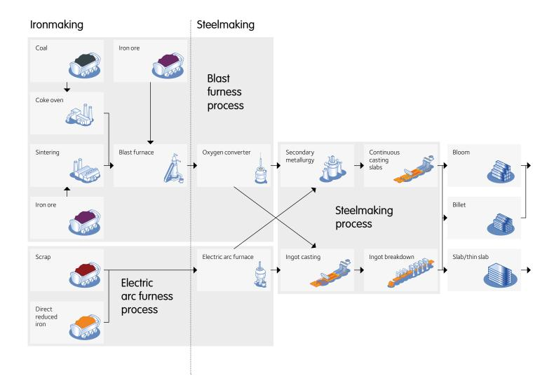
Steel is produced from iron ore or scrap. Iron ore is a mineral aggregate that can be converted economically into iron. The quality of the iron ore is mainly determined by its composition: a high iron content and low sulphur and phosphorus contents are favorable. Iron ore can be found all over the world, but its iron content varies.
